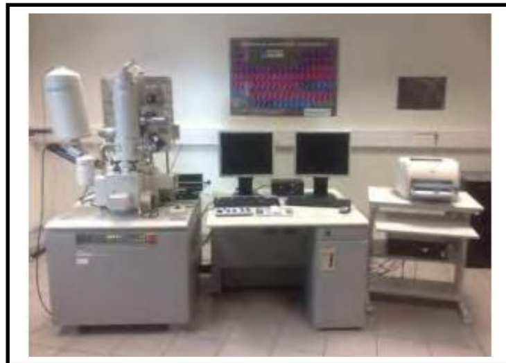
Figure II.13 : Image du MEB de type FEI Quanta 450 FEG.
