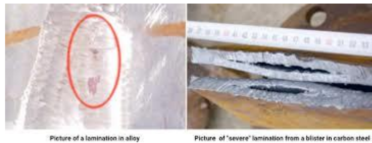
Figure I. 18. Picture of a lamination defect
