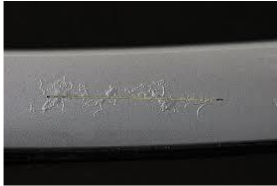
Figure I. 22 Defect under coatings
