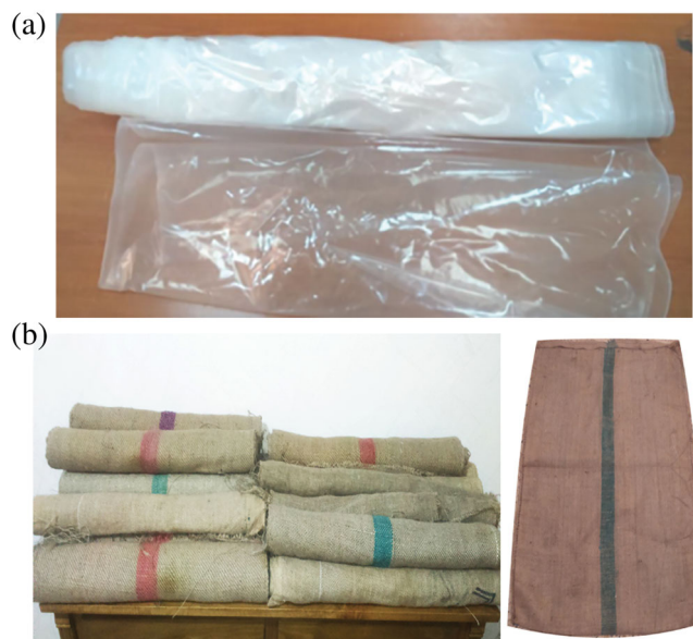
FIGURE 1 Constituents used in the development of biocomposites: (A) polypropylene film and (B) jute bags
