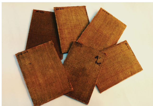
FIGURE 2 Plates from the composite jute-polypropylene
