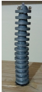
Fig. 5.9: A section of the continuum robot design with a novel ball disk [19]
