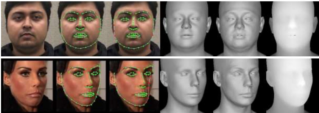
Figure 30: the predicted 2D landmarks, 3D landmarks (red means non-visible points), coarse geometry, detailed geometry, and depth.
