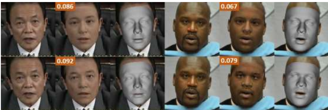
Figure 40: Comparison of the results with only image-level losses (top row) and with both image-level and perceptual losses (bottom row) for training.
