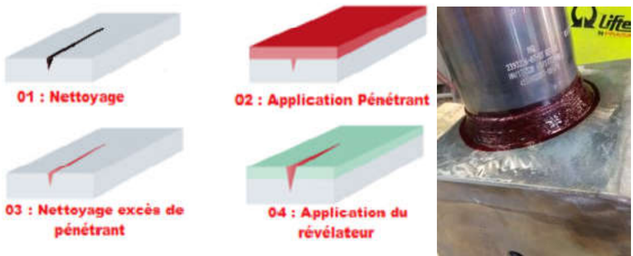
Figure I. 2– Principe du ressuage [1].
