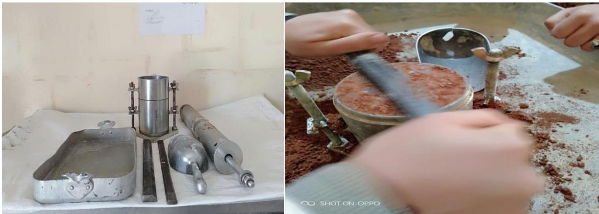
Figure II-8: Appareil essai Proctor normal.
