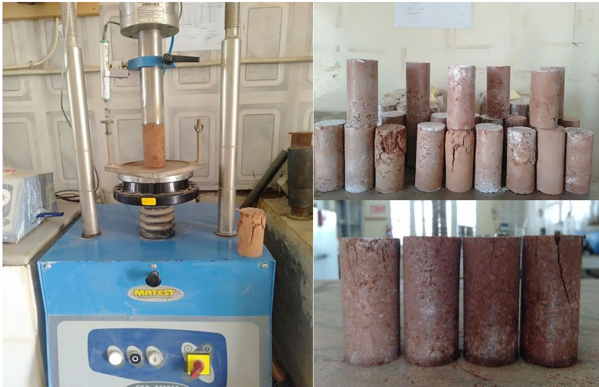
Figure II-10: Essais de compression simple.
