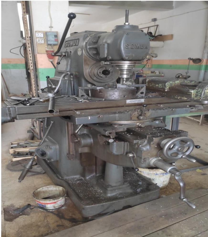
Figure III.2: Fraiseuse universelle .H.ERNAULT-SOMUA TYPE Z 3C
