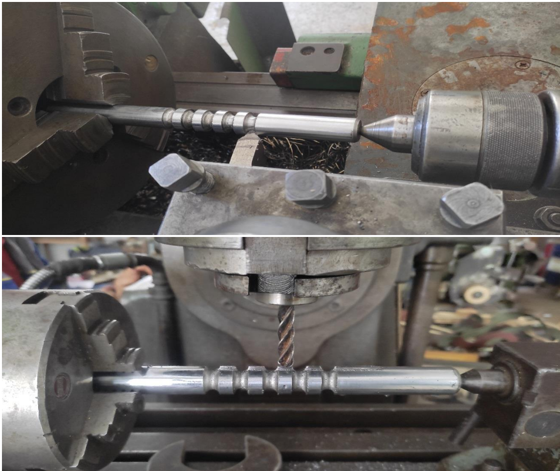
Figure III.8: usinage du coulisseau
