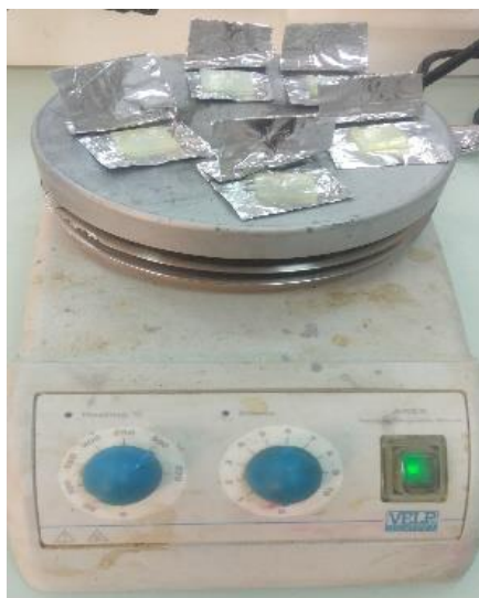
Fig. IV.5: Hot plate used to dry the obtained samples.
