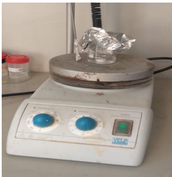
Fig. IV.2: Solution refluxing and stirring at 60°C.
