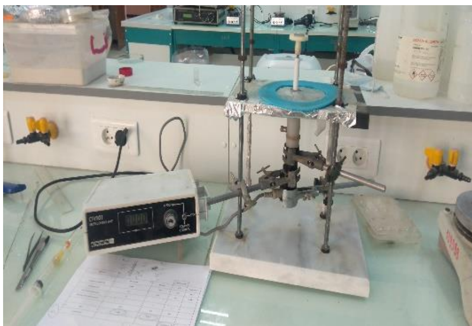
Fig. IV.4: Spin-coating system used to deposit S-doped ZnO samples.
