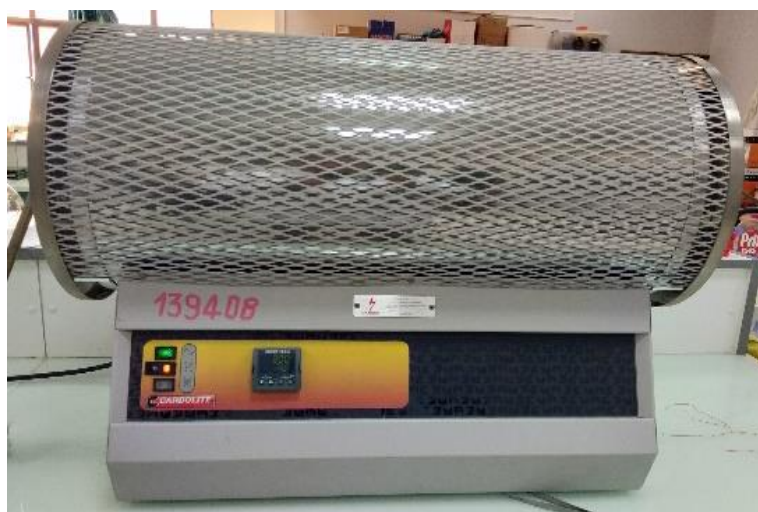
Fig. IV.6: Carbolite high-temperature tube Furnace used to anneal the S-doped ZnO obtained samples.
