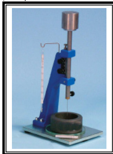
Photo. II.3 Appareil de VICAT [39]
