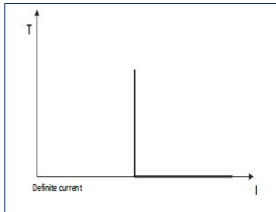
Figure 29 : Definite current "instantaneous" overcurrent relay Curve
