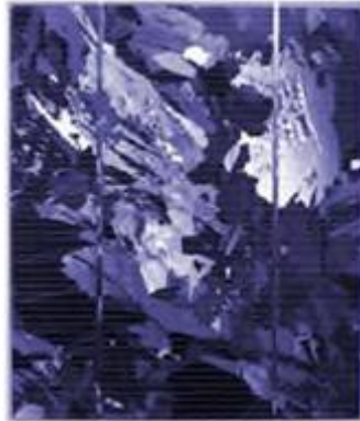
Figure 1.13 Photo de cellule poly cristallin.
