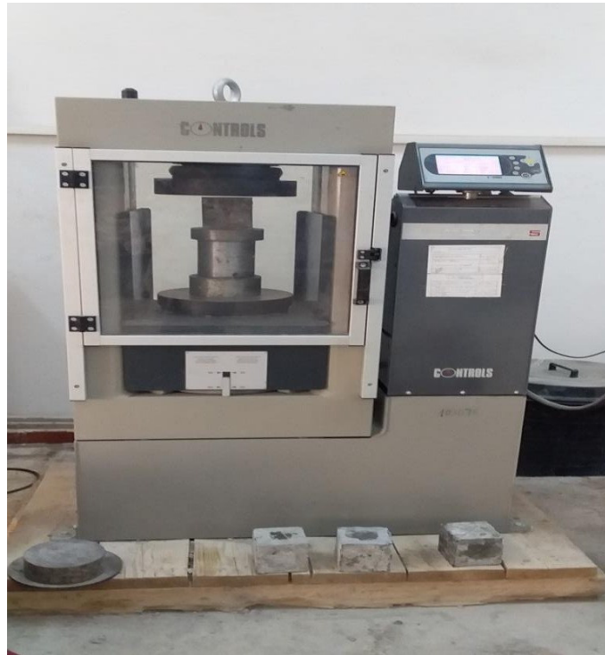
Figure III.25: Machine d'essai de compression.
