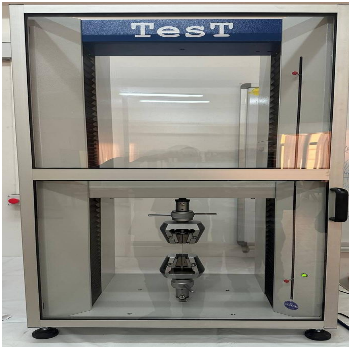
Figure III-25: La machine de test traction
