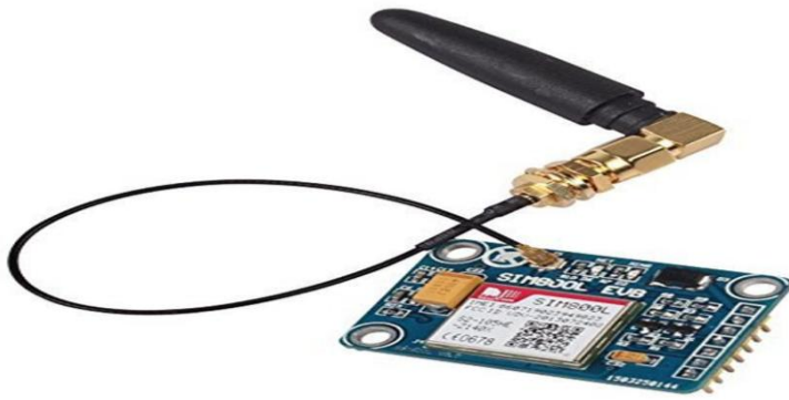
Figure IV.11: Le module SIM800L
