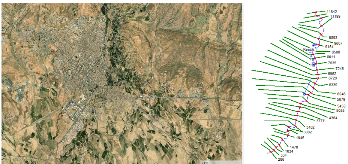
Fig. 3.20 Satellite imagery of M'sila city (to the left) and downstream K'sob reach geometry in HEC-RAS (to the right)
