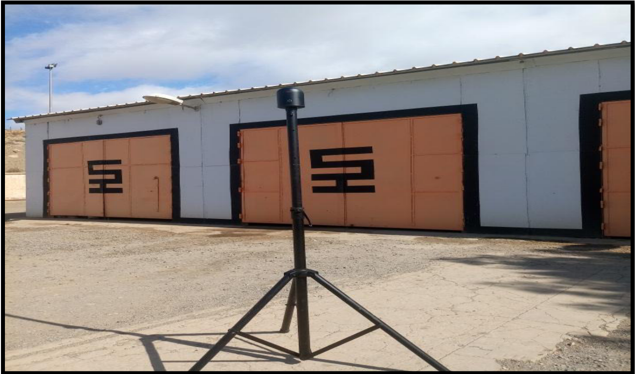
Figure 35 : Le scanner 3D Leica BLK360
