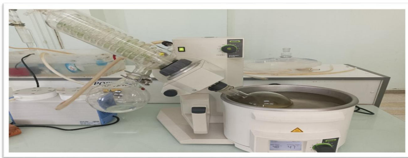
Figure 18. Device of the rotary Rota-steam type (BÜCHI R- 120) (Maalem N., 2023).
