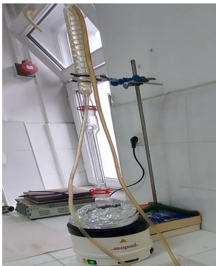
Figure 21. Original hydrodistillation photo of clevenger type (Maalem N., 2023)
