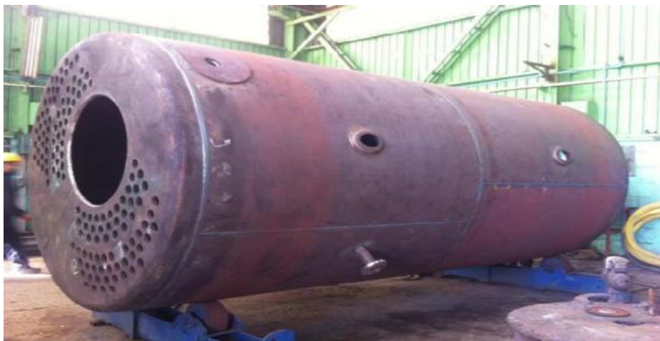
Figure IV.8. Shell with tube plates and spigots [1].
