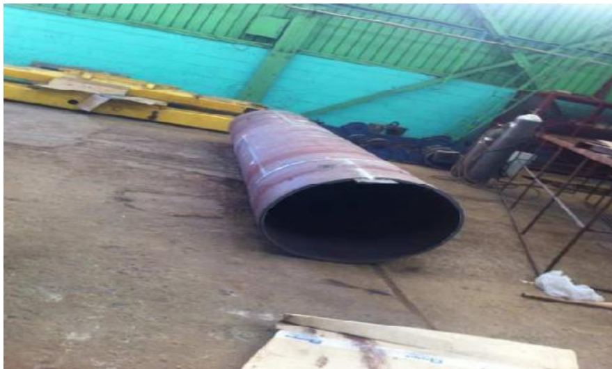
Figure IV.6. MYRA4000 smooth focus tube [1].
