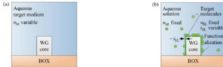
Figure 12: Plain and functionalized strip WG on a buried silicon oxide (BOX) layer. (a) Homogeneous sensing. (b) Surface sensing [29].
