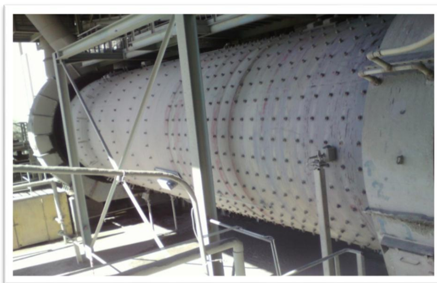
Figure I-9 : Broyage ciment (horizontale).
