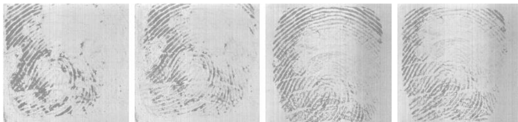
Fig. 2.6 fingerprints' failure to enroll caused by poor quality ridges due to extreme finger dryness [3]
