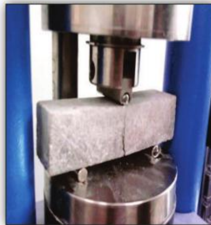
Figure IV. 9 Essai de flexion.
