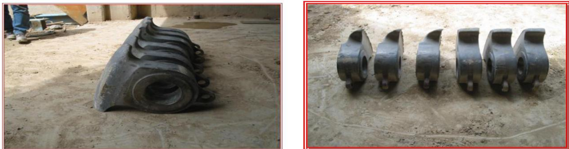
Figure. II.17: Usure rapide des marteaux Mg 12%
