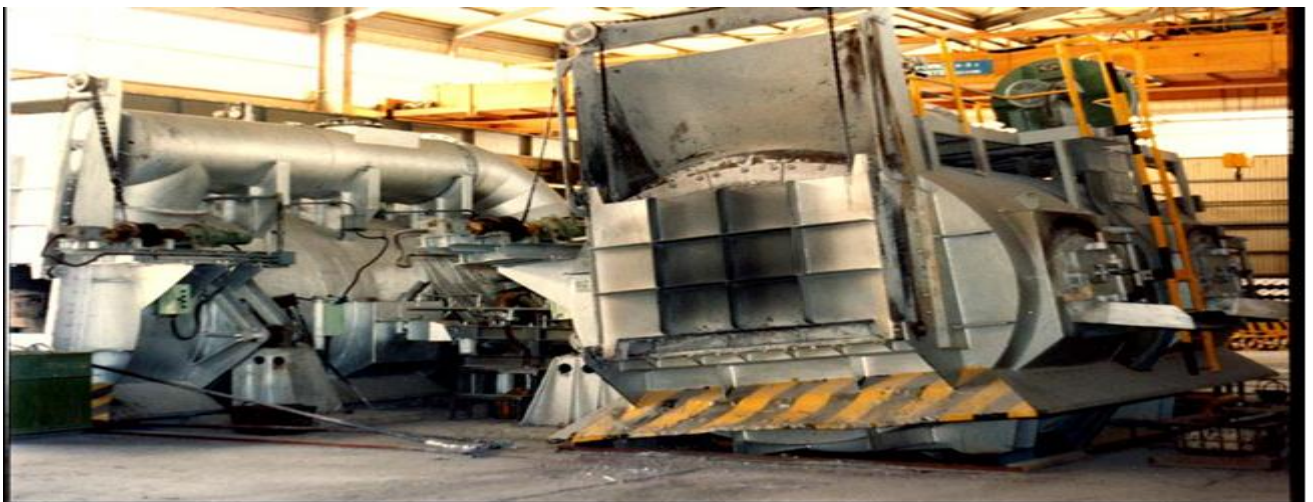
FIGURE I. 4. FOUR DE FUSION.
