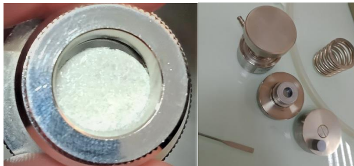
Figure (II.2) A thin sample placed in a special holder for studying with the device and means of pressure.
