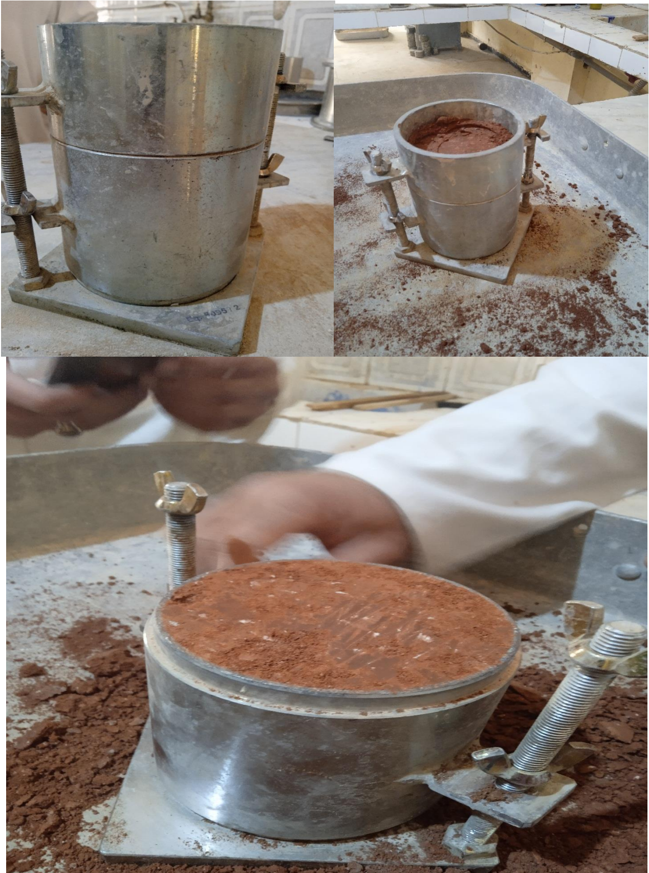
Figure : II.8 Essai Proctor
