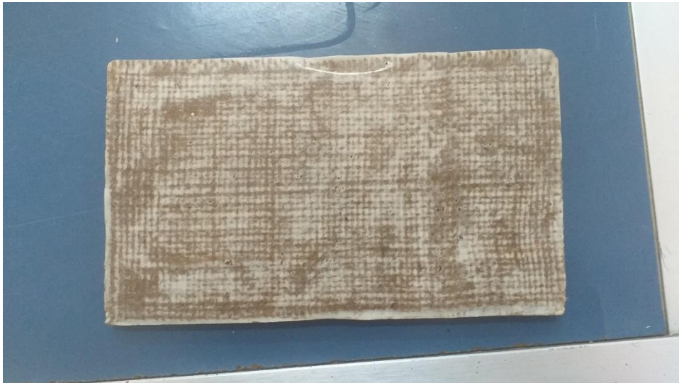
Figure III-8. Plaque composite renforcée (10 % alumine)
