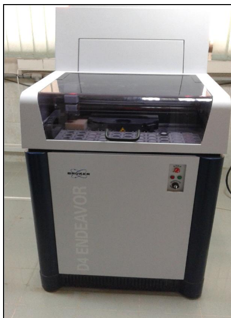
Figure 3-10 DRX BRUKER D4 ENDEAVOR ( Lafargeholcim laboratoire )
