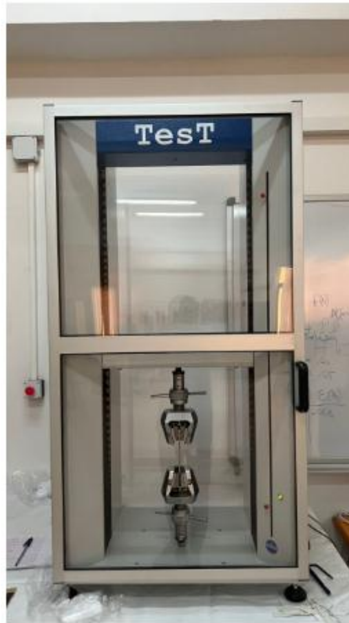
Figure.II. 8: Machine de traction TEST.
