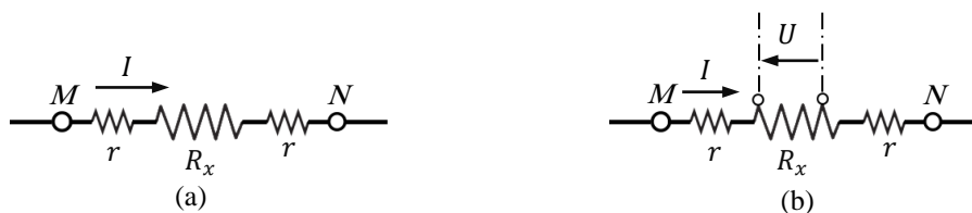
Figure 2-11: (a) Equivalent diagram of a real resistor (b) Four-terminal resistor
