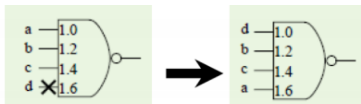
Figure 15: Pin swapping applied on a NAND gate
