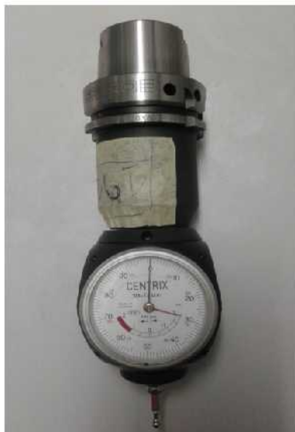
Figure II.11: Palpeur 3D de la marque "Mitutoyo"
