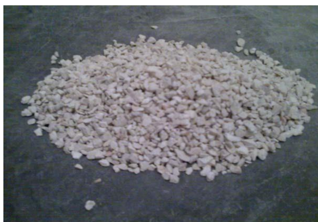
Figure III.11 Gravillon 3/8 (carrière ENG)
