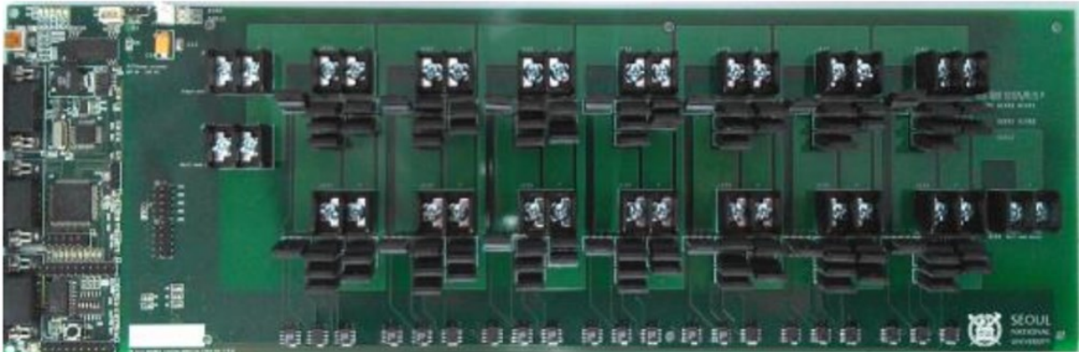
Figure 38 Computer-controlled programmable switch board.
