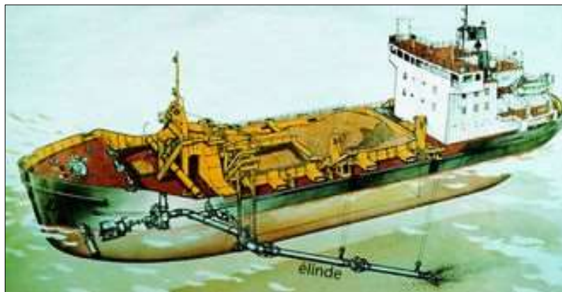
Figure II.13: Dragues aspiratrices simpl.
