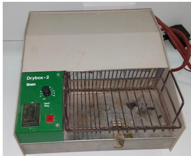
Figure IV-13. Séchoir air chaud
