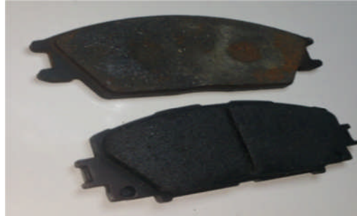
Fig. II.12 : Usure excessive des plaquettes
