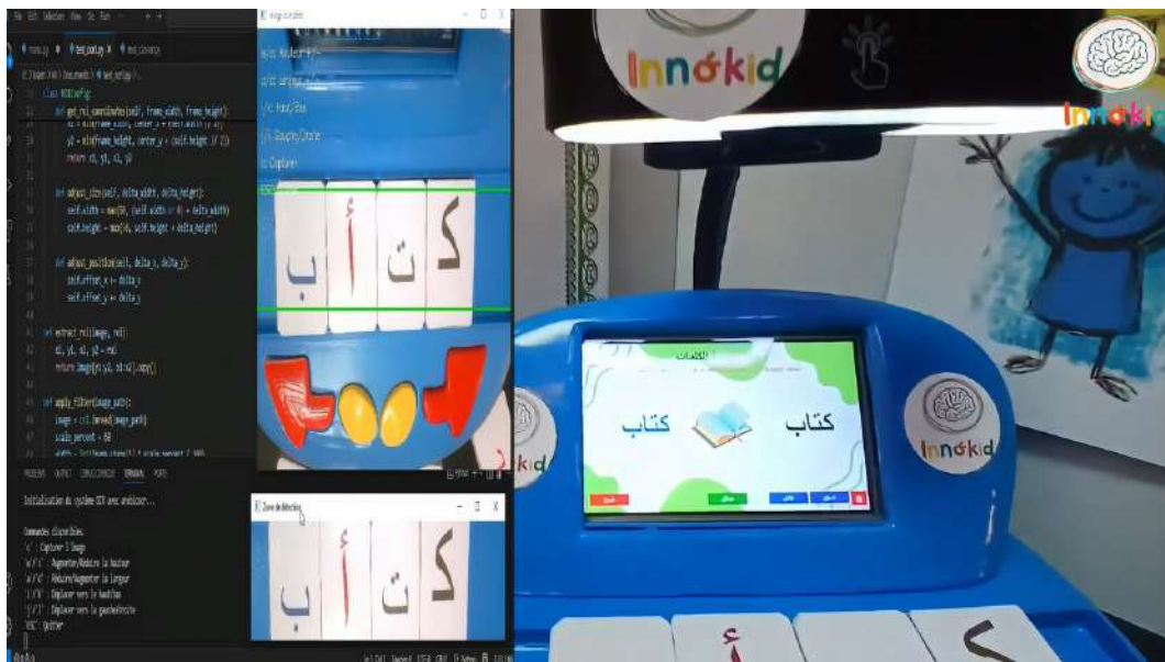
Figure 3.5: Illustration of the real-world operation of the InnoKid interactive system with visual letter recognition.
