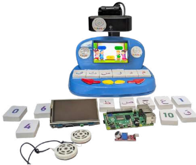
Figure 3.14: Functional prototype of the InnoKid interactive educational device utilizing camera vision and physical interaction
