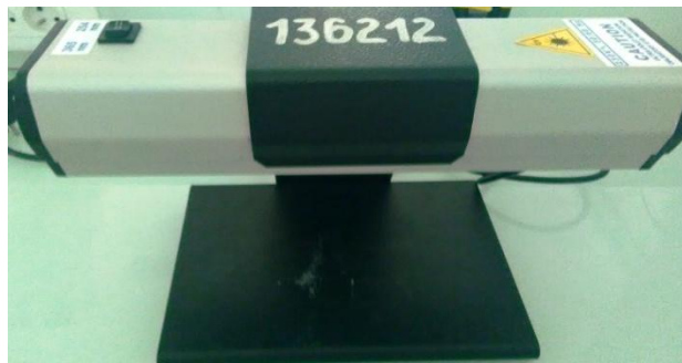
Figure 13 : Lampe Ultra –Violet 254 – 365 nm.
