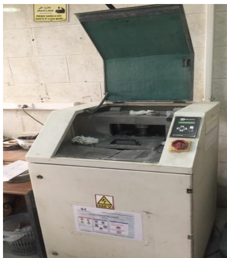
Figure 27: Presse manuelle de pastilles.
