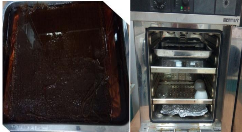
Figure. III.8 : Imprégnation des tissus (Solution 5% NaOH / 2 H
