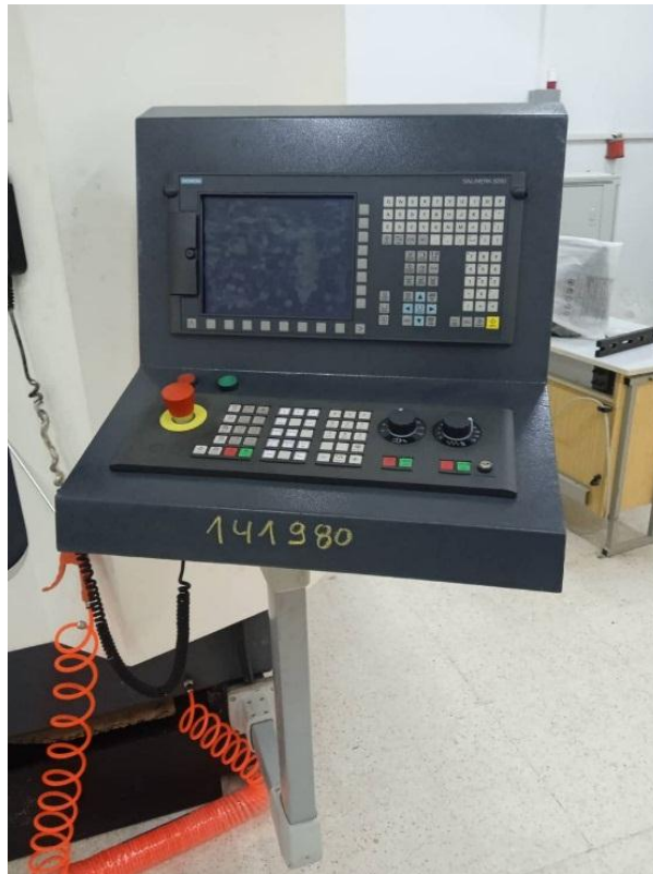
Figure II.7 : interface de programmation SINUMERIK 828d
