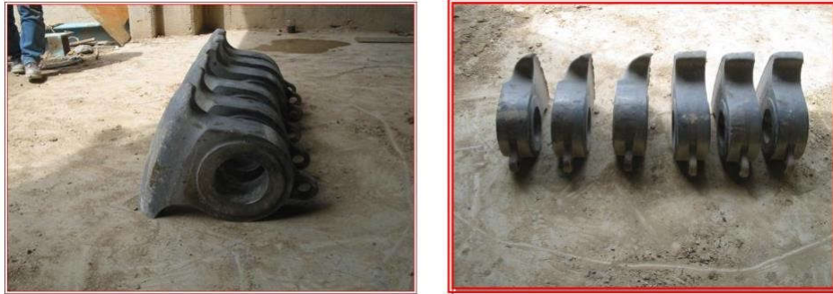
Figure 3. 14: Usure rapide des marteaux Mg 12%.
