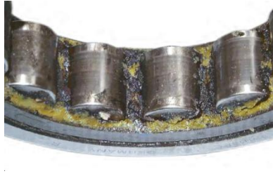
Fig I. 20 Lubricant degradation Black discolored grease on the cage bars caused by passage of current
