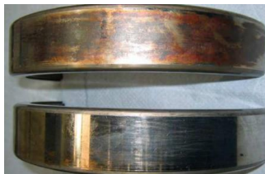
Fig I. 19 Fretting corrosion on the outer diameter of a bearing
