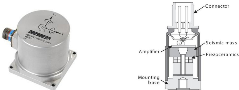
Fig I. 11 Principle diagram of an accelerometer.
