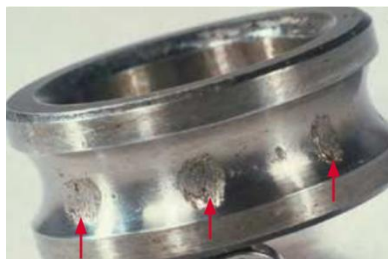
Fig I. 21 The dents, resulting from wrong mounting, are overrolled and quickly lead to spalls
